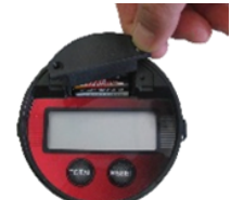
Figure 4: Step 4: Insert the battery cover, then screw the battery cover tight
